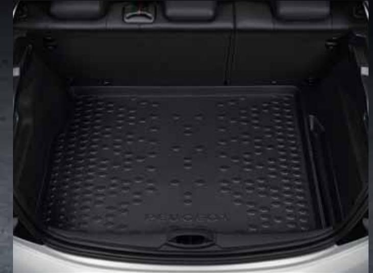
**Soft thermoformed boot tray**
